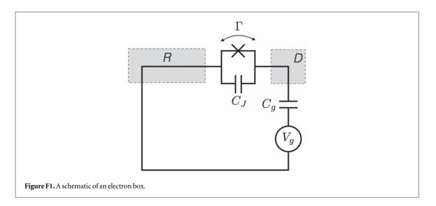
The system (figure F1) consists of a large metallic electrode R that serves as a charge reservoir, a small metallic island (or quantum dot) D, and a gate electrode. The island D is coupled only capacitively to the gate electrode but couples to the reservoir R capacitively and via tunneling. The Hamiltonian has four parts:  $H = H_R + H_D + H_C + H_T$ . The first two terms,
