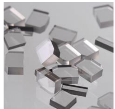
Type IIa diamond: ~ 1 ppm [N] Electronic grade: < 5 ppb [N]
