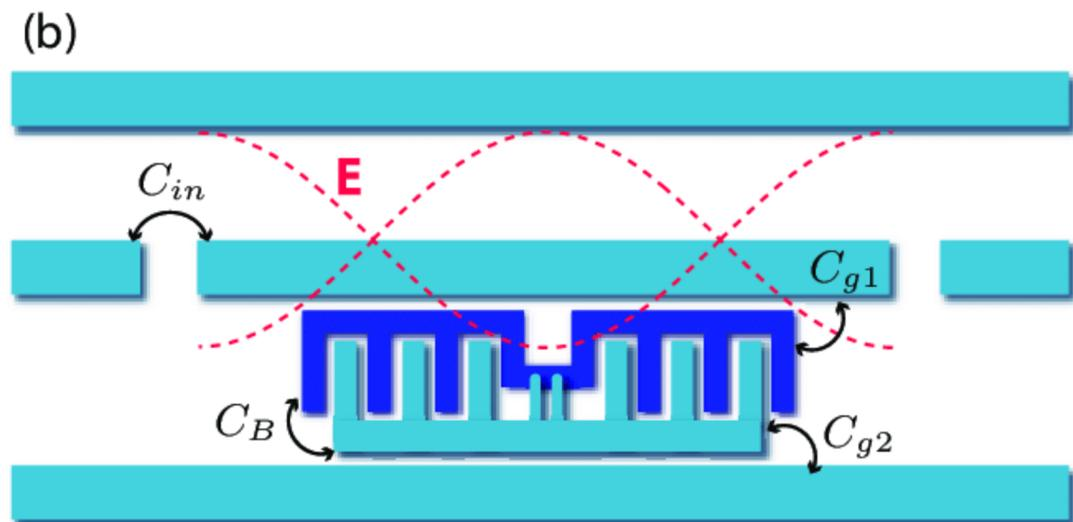
$$H = \underbrace{E_C (n - n_g)^2}_{\text{perturbation}} - E_J \cos \phi$$
