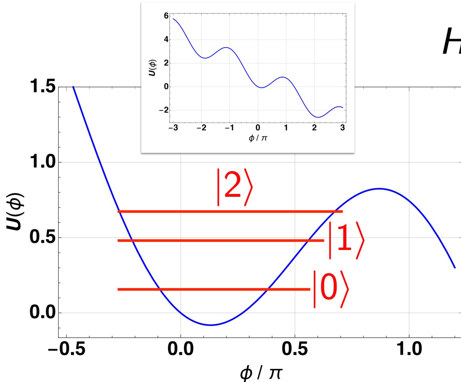
$$H = \underbrace{E_C(n - n_g)^2}_{\text{perturbation}} - E_J \cos \phi - I\phi$$
