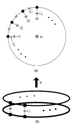
FIG. 1. Schematic diagrams of (a) a single Josephson-junction necklace (from above) and (b) two capacitively coupled necklaces (from the diagonal direction). In (b) each thick ring represents the single necklace depicted in (a).
